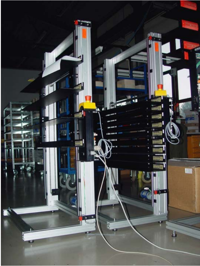
In this picture, two extremes can be seen in relation to the different track sizes: The LokLift on the left is a four-level version for gauge 1, the one behind it is one with nine levels for Z gauge.
