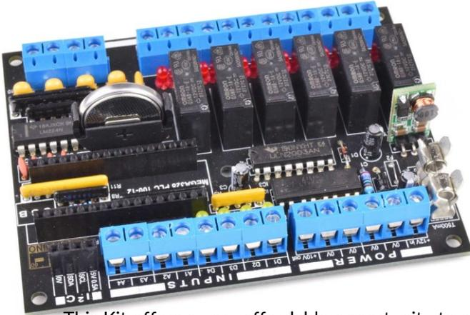
**CANADUINO MEGA328 100-12 PLC** is built around an Arduino NANO V3.0 module (or compatible) and can be programmed using Arduino IDE or visual programming using for example Mitov’s awesome “Visuino” software.
