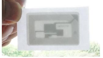
*It also supports reading flexible tag. We tested flexible tags of Mifare 1 S50 and Ultralight. The reading distance is up to 5cm.*
