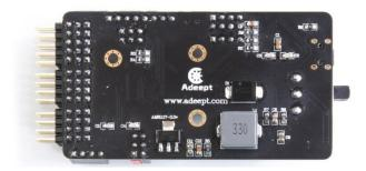
[Vin]: it is an interface for external power supply, range: 6-24V.
